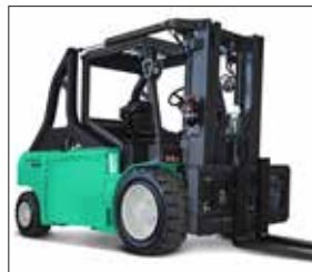
Low overhead guard for container applications.
